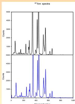
The response function of SiPIN detectors is not reported in the literature and cannot be compared its performance with the other detectors. We have studied it and two commercially available detectors' spectra are presented for the 241Am source.
