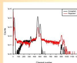
The two spectra, accepted and rejected, for an 55Fe source. The line shape of the x-ray lines are reasonably good. It has merit for application.
