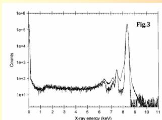
The response function of a high-quality HPGc detector at 8.46 keV x-ray energy. The spectra were measured at 10 (upper curve) and 80 (lower curve) microseconds processing times with the same signal processor, otherwise under identical conditions. The peak-like structures between 6 and 8 keV are identified as Ge L-shell x-ray escape peaks, and Auger and photoelectron peaks of detector and front contact materials.
