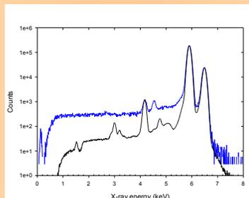
Spectra of 55Fe sources measured with silicon drift detectors and two different signal processors. The tailing cannot be attributed to a dead layer in this case. The spectrum with black line presents several expected features.
