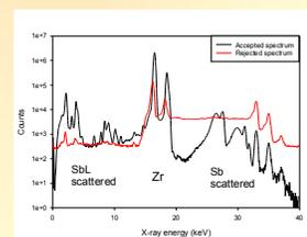
Measurement with a trapezoidal noise filter was selected as a compromise, sacrificing some energy resolution, but having a simpler rejected spectrum. Here the continuous pile up plateau is flat, and the ghost peak is in the rejected tail spectrum.
